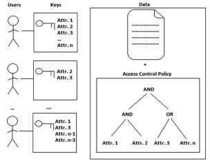
Figure 2. Ciphertext-policy attribute-based encryption
