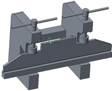
Figure 2: Modeling of available hand press brake
