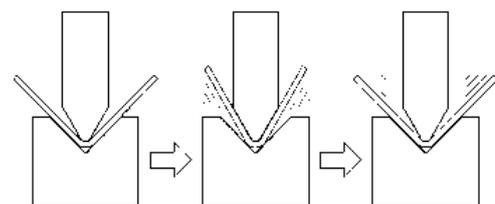
Figure 1: Air bending
