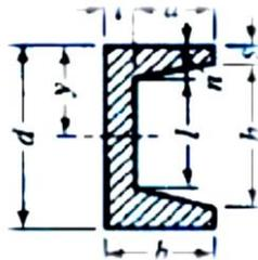
Figure 3: C-channel section
