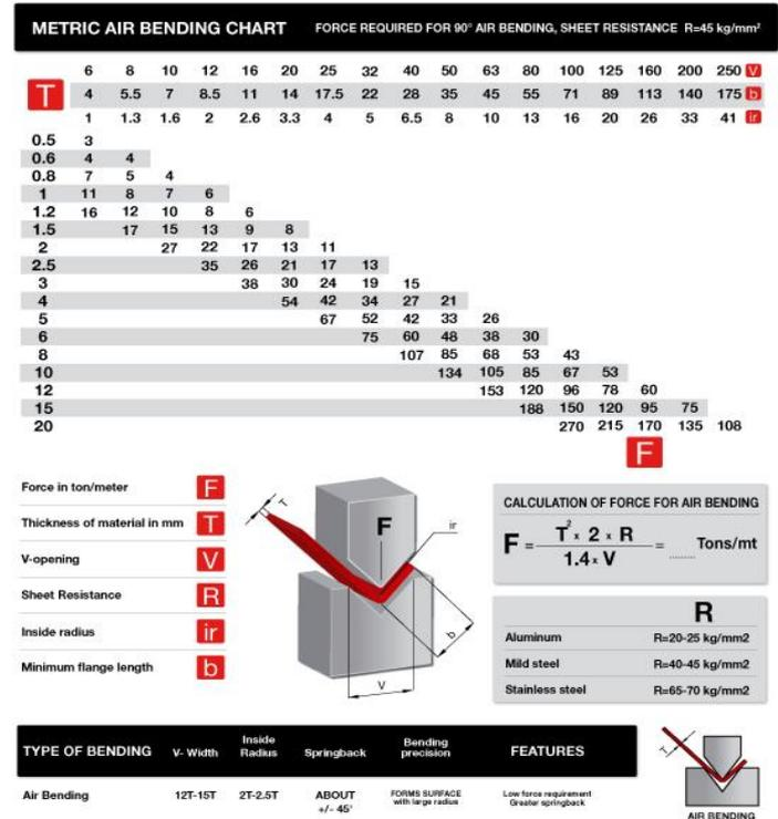
Figure 4: Metric air bending chart [1]
