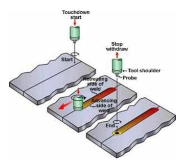
Figure 1. Friction Stir Welding
