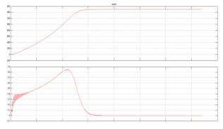
Figure 6. Speed and Torque of I.M with Module Model
