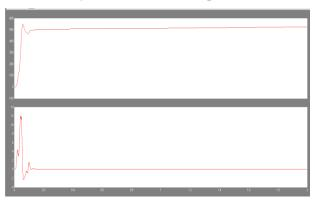
Figure 8. Speed and Torque of I.M with PI controller with Module Model (Base speed 500 RPM)
