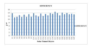
Figure 3. Efficiency of Solar Tunnel Dryers
