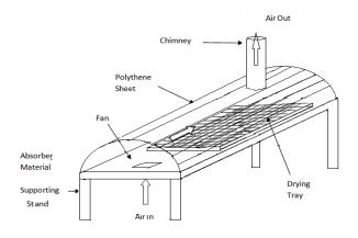
Figure 1. Schematic of Solar Tunnel Dryer
