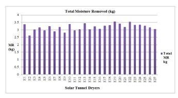
Figure 4. Total Moisture removed from chillies
