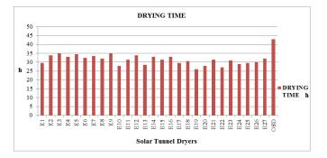
Figure 5. Variation in drying time for dryers
