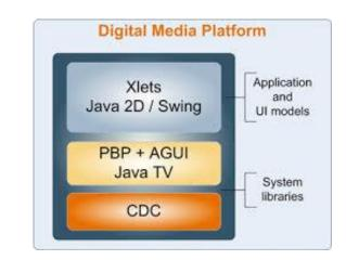
Figure C: The Connected Device Configuration (CDC)
