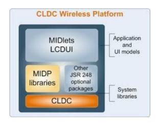
Figure B: The Connected Limited Device Configuration (CLDC)
