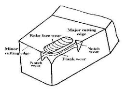
Figure 2: Rack Face and Flank Face
