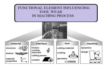
Figure 1: Elements Affecting Tool Wear
