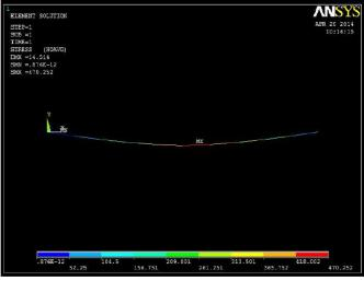
Figure 7. Stress plot of SSB (T Cross-section)
