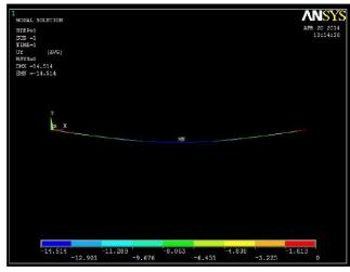
Figure 6. Deflection of SSB (T Cross-section)
