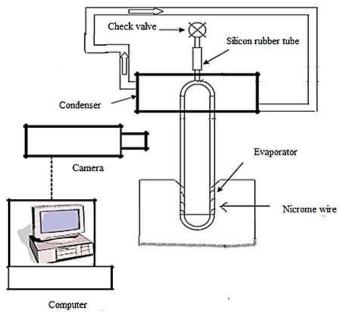
Figure 3. Experimental layout of CLPHP
