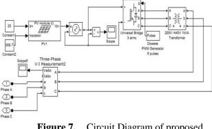
Figure 7. Circuit Diagram of proposed STATCOM
