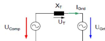
Figure 3. Single Line Grid Connection
