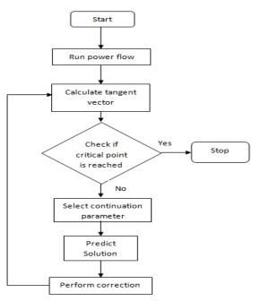
Figure 2 : Flow Chart for Continuation Power Flow [20]
