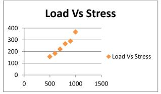
Graph 4: Load Vs. Stress for New Spring
