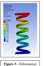
Figure 3:- Deformation 1000 N Load
