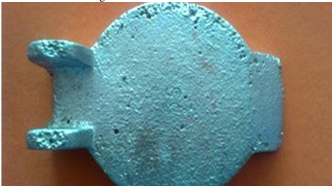
Figure 12. Defective Casting from Experimental Trial 9 showing rough surface finish, gas holes and sand inclusion
