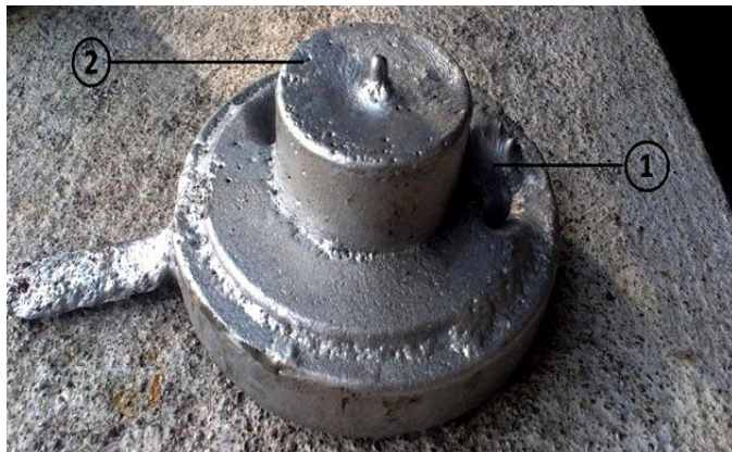
Figure 6. Defective Casting from Experimental Trial 3 showing shrinkage porosity and metal sinking
