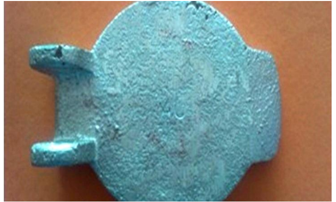
Figure 9. Defective Casting from Experimental Trial 6 showing rough surface finish and sand inclusion
