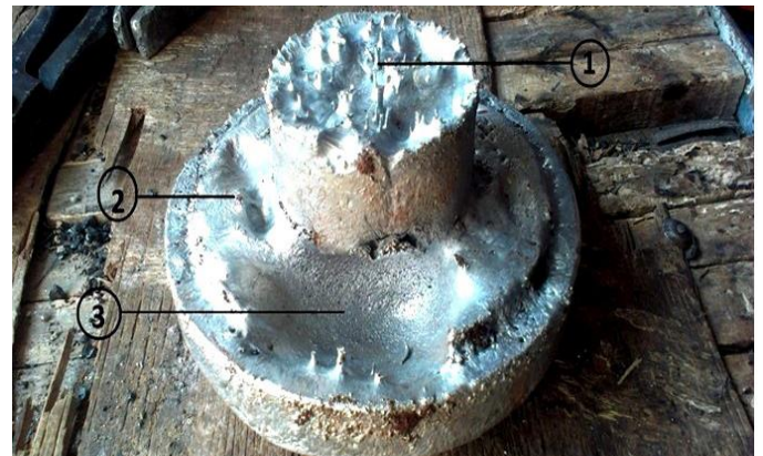
Figure 5. Defective Casting from Experimental Trial 2 showing shrinkage porosity and metal sinking defect.
