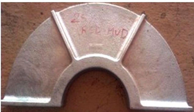
Figure 14. Sound Casting from Experimental Trial 10 with 25% red mud showing a better acceptable surface finish
