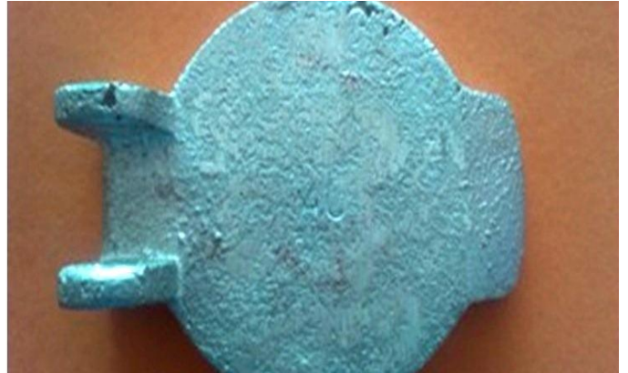
Figure 11. Defective Casting from Experimental Trial 8 showing rough surface finish and sand inclusion and pin holes
