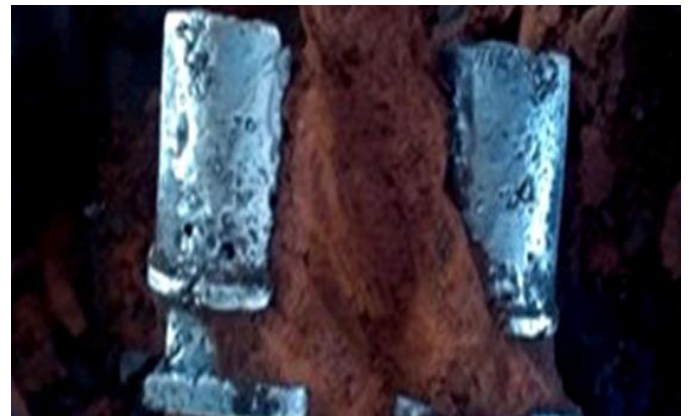
Figure 5. Defective Casting from Experimental Trial 2 showing shrinkage porosity and metal sinking defect.
