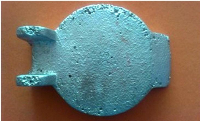
Figure 10. Defective Casting from Experimental Trial 7 showing rough surface finish and sand inclusion
