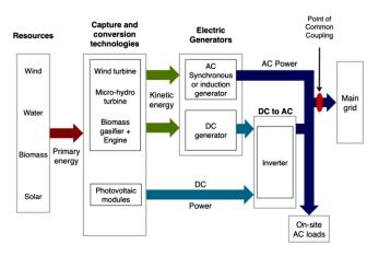
**Figure 2.** Energy pathways in a renewable power minigrid connected with the utility grid<sup>[17] [</sup>2013].
