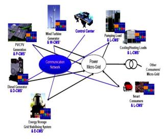
Figure 1. Major Components of a Microgrid System
