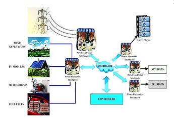
Figure 3 : Power electronics interface in a Micro-grid
