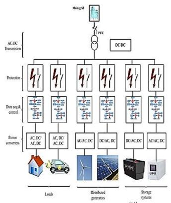
**Figure 3.** Micro-grid Distribution Model<sup>[11]</sup> with DGs, DERs, interconnected micro-grids, and ICT.
