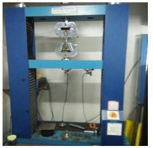
Figure 3. Universal testing machine with test piece
