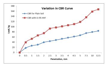
Figure 4: CBR Values with and without reinforcement of HHF
