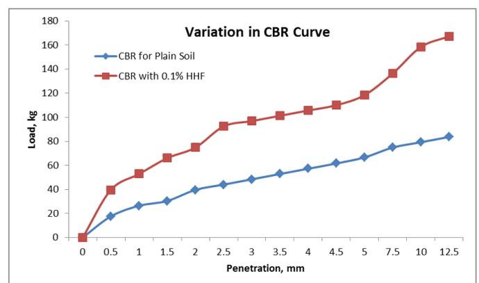
Figure 4: CBR Values with and without reinforcement of HHF
