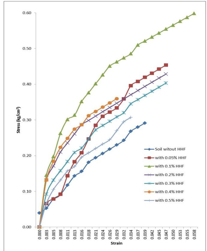
Figure 2: UCC curve for varying percentages of HHF
