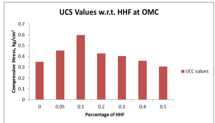
Figure 3: Variation of strength with varying percentage of HHF
