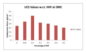
Figure 3: Variation of strength with varying percentage of HHF
