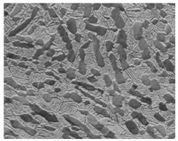
Figure 2.2. Photomicrograph of DP steel
