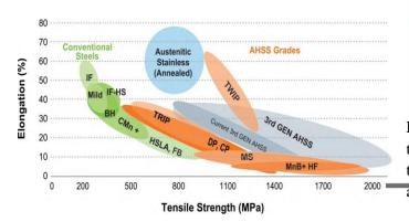
**Figure 1.** Global formability diagram, illustrating the range of properties available from today's AHSS grades (WorldAutoSteel, 2014).
