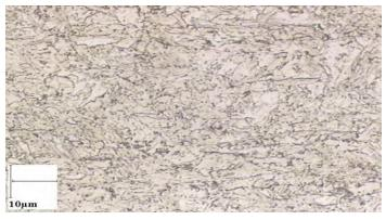
Figure 2.8 : Photomicrograph of CP 800/1000 hot rolled steel.
