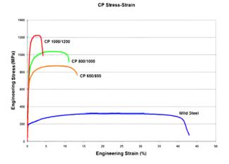
**Figure 2.9 :** Engineering stress-strain curves for a series of CP steel grades.V-1 Sheet thickness: CP650/850 = 1.5mm, CP 800/1000 = 0.8mm, CP 1000/1200 = 1.0mm, and Mild Steel = approx. 1.9mm (International Iron and Steel Institute, 2006).
