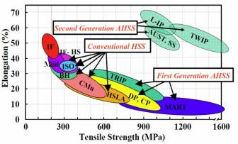
**Figure 2.** Relationship between tensile strength and total elongation (50.8mm gauge length) for various types of steel (r/t) for various AHSS (International Iron and Steel Institute, 2006)
