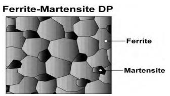
Figure 2.1: Schematic shows islands of martensite in a matrix of ferrite
