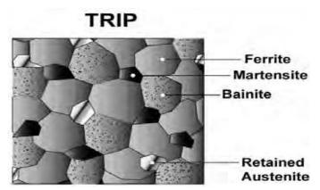
**Figure 2.4 :** Bainite and retained austenite are additional phases in TRIP steels
