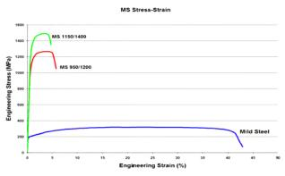
Figure 2.7 : Engineering stress/ strain curves for various type of MS steel grades
