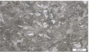
Figure 2.6: Microstructure for MS 950/1200
