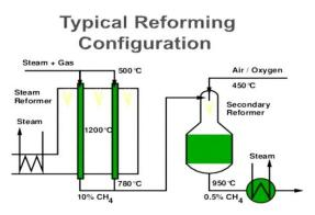
Figure 1. Typical Reforming Configuration.
