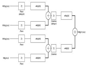
Figure 3. Inverse DWT Process
