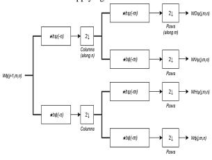
Figure 2. DWT Process
