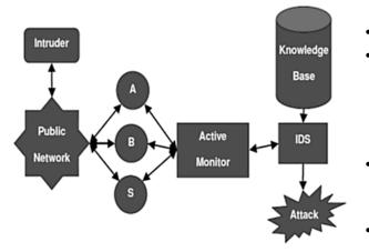
Figure 4. Architecture of IDAODV
