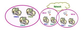
**Figure 1.** Ad Hoc and Infrastructure Network Topologies
