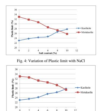
Fig. 5: Variation of Plastic limit with MgCl<sub>2</sub>
