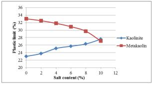
Fig. 6: Variation of Plastic limit with CaCl<sub>2</sub>
