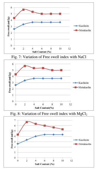
Fig. 9: Variation of Free swell index with CaCl<sub>2</sub>
