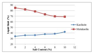
Fig. 2: Variation of Liquid limit with  $MgCl_2$
