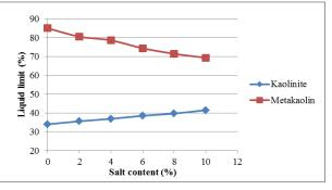
Fig. 3: Variation of Liquid limit with CaCl<sub>2</sub>
