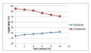
Fig. 1: Variation of Liquid limit with NaCl
