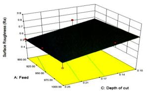
Chart-2 (c): Response Surface at C.S of 3900 RPM
