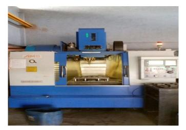
Figure 1. CNC Vertical Machine Center
