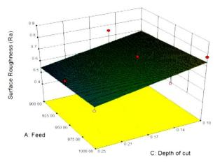
Chart-2 (b): Response Surface at C.S of 3500 RPM
