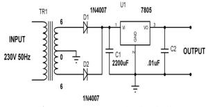
Figure 7. Power supply circuit diagram
