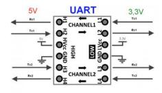
Figure 6. UART Pin Configuration
