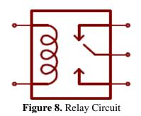
The input circuit is switched off and no current flows through it until something (sensor) turns it on. The output circuit is also switched off.
