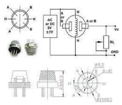
Figure 4. The MQ4 gas sensor.
