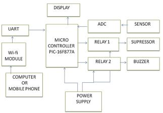
Figure 2. Block diagram of user interatactive toxic gas suppressor system.
