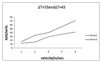
**Figure 1.** Variation of h under various  $\Delta T$  conditions for steel
