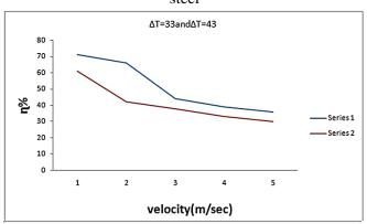
Figure 3. Variation of  $\eta$  under various  $\Delta T$  conditions for aluminium
