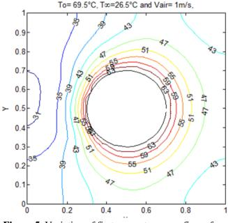
Figure 5. Variation of fin temperature over fin surface for 1m/sec velocity for  $\Delta T=43$  °C
