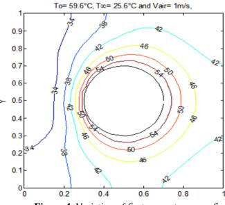
**Figure 4.** Variation of fin temperature over fin surface for 1m/sec velocity for  $\Delta T=33^{\circ}C$
