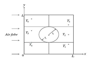
Figure 2. physical geometry of two-dimensional plate fin with a circular tube
