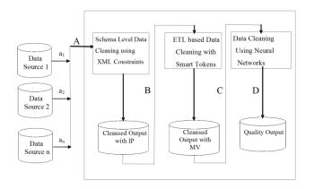
Figure1.An ECDC Framework for Data Cleaning
