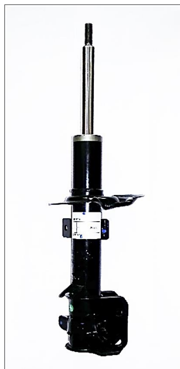
Figure 1: Test Specimen -Front Damper
