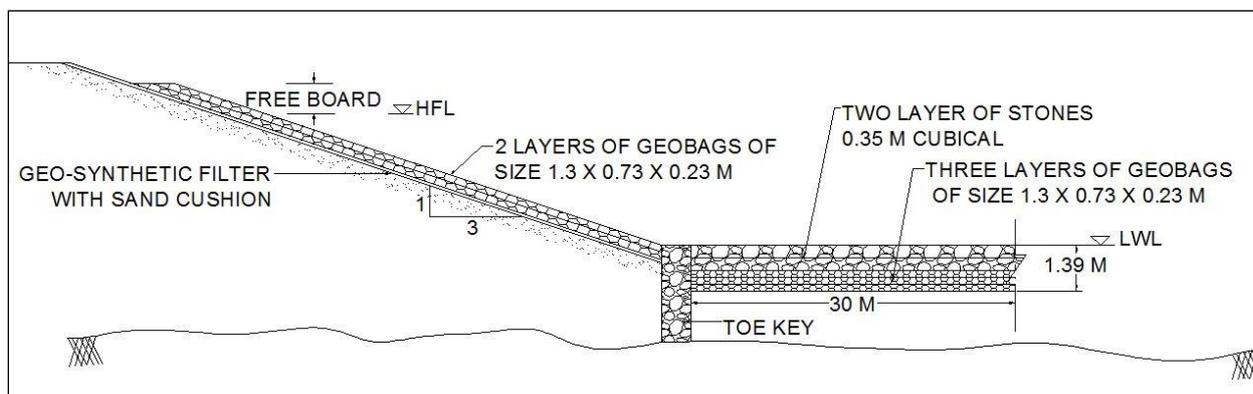
**Figure 9:** Final design adopted for the protection work of study area
