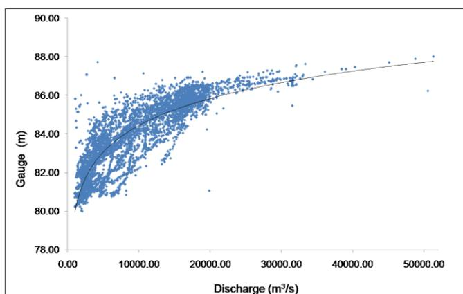
**Figure 6 :** Gauge Discharge curve used for downstream boundary
