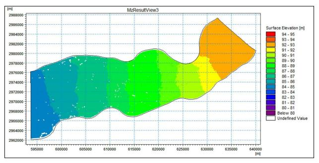
Figure 7: Water Surface Profile for a discharge of 50,000 m<sup>3</sup>/s
