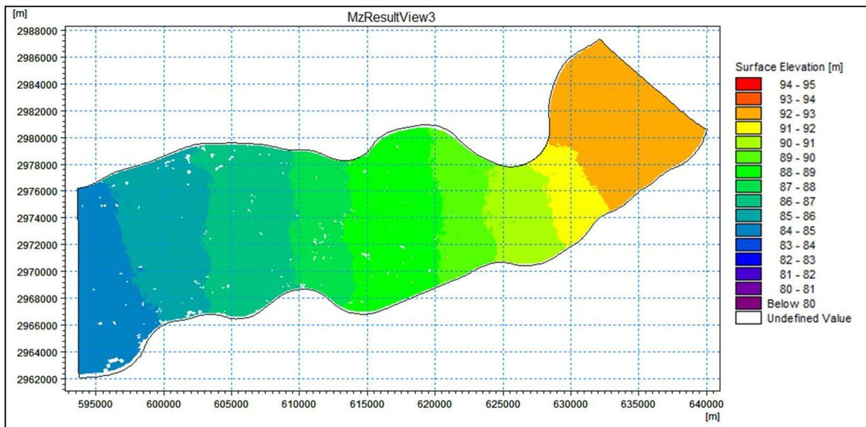
Figure 7: Water Surface Profile for a discharge of 50,000 m<sup>3</sup>/s
