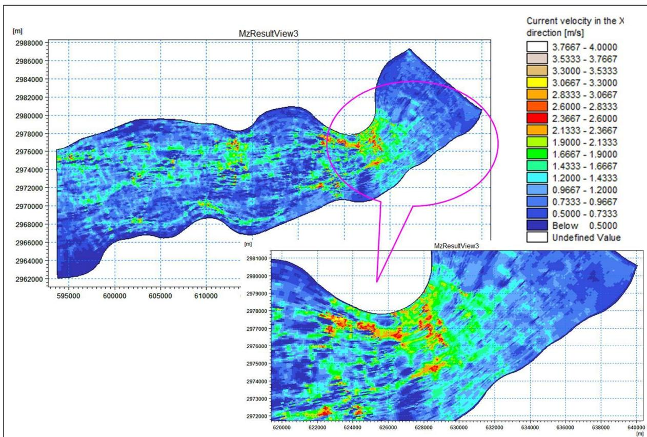
Figure 8: Velocity Profile for a discharge of 50,000 m<sup>3</sup>/s
