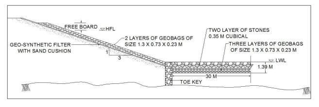
Figure 9: Final design adopted for the protection work of study area
