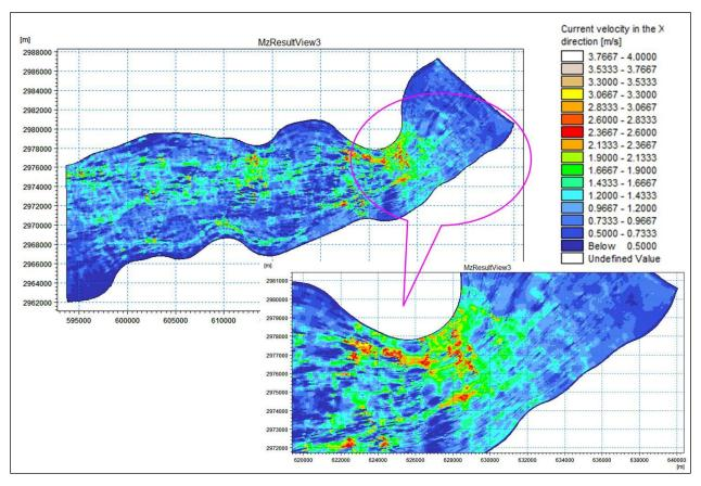
**Figure 8**: Velocity Profile for a discharge of 50,000 m<sup>3</sup>/s
