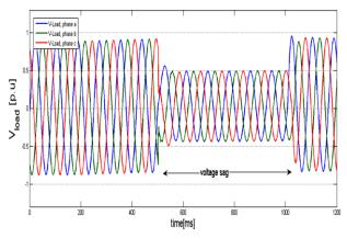
Figure 7. Three-phase load voltage sag waveform
