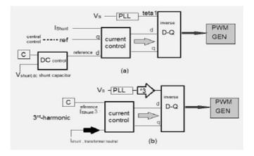
**Figure 6.** The shunt control configuration: (a) for fundam ental frequency (b) for third-harmonic frequency
