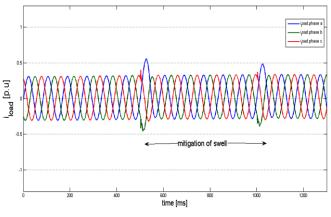
Figure 10 : Mitigation of three-phase load current swell with DPFC
