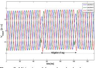
Figure 8: Mitigation of three phase load voltage sag with DPFC
