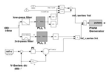
Figure 5. Block diagram of series control structure in Matlab/Simulink
