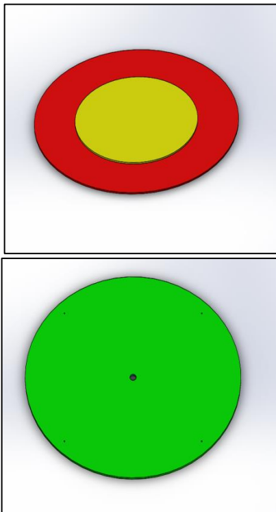
Figure 2.7: (a) Assembly of Vibrating Plate + PZT; (b)Separator Plate
