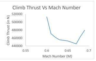
Figure 8 : Variation in climb Thrust at different Mach Number
