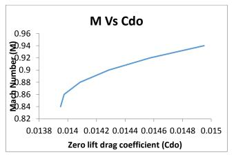
Figure 3 : Variation in zero-lift drag at different Mach Number
