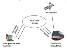
Figure 1. Schematic Overview of Automated System
