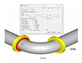
Figure 6: Value of torsional stiffness for flexible joints is considered as 165839.02Nm/deg
