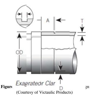
• Rolled Grooves: The rolled groove profile presses/ rolls the profile into the pipe and no material is lost. There is a potential for a small amount of deformation and thinning through the profile of the groove. This potential for thinning has been reviewed against the recommended pipe wall thickness and there is enough additional material to permit an amount of thinning and still meet the full design pressures required for the utility systems.
