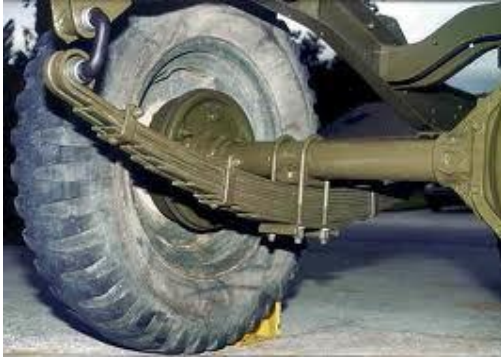
Figure 2 : Steel Leaf Spring used in Vehicles (e.g. used in trucks)
