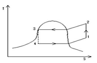
Figure 1 : Temperature-entropy diagram of the cold room storage cycle processes
