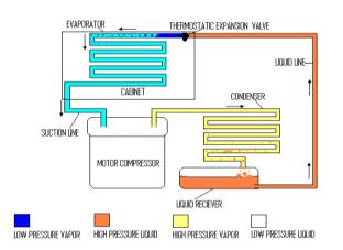
Figure 2 : Processes of refrigeration employed in the cold room
