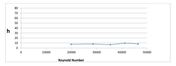
Figure 10. Effects of Reynolds number on Heat transfer Coefficient with series connection
