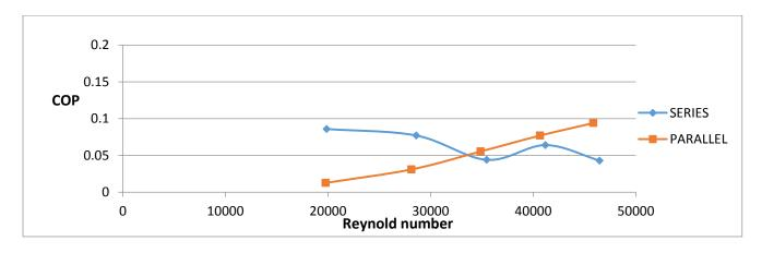
Figure 15. Comparison of COP vs. Reynolds number for both connections
