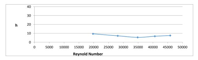
Figure 7. Effect of Reynolds number on Heat transfer Coefficient
