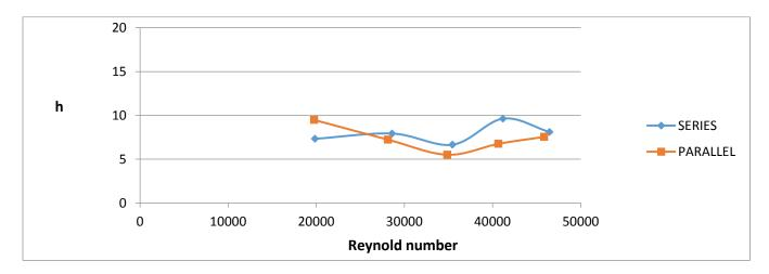
Figure 13. Comparison of heat transfer coefficient vs. Reynolds number for both connection
