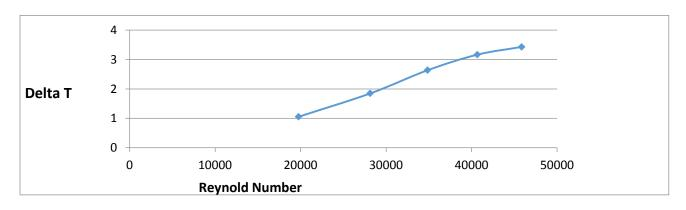
Figure 8. Effect of Reynolds Number on Temperature Difference
