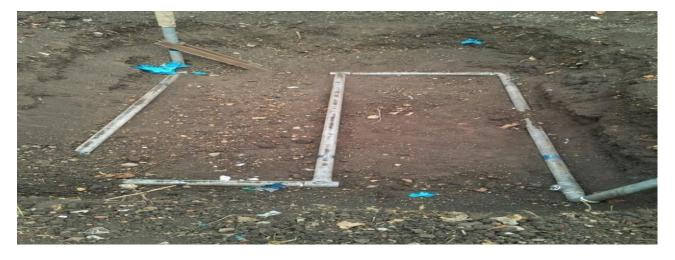
Figure 5. Experimental setup in series connection (2.5 inch diameter) without covered soil
