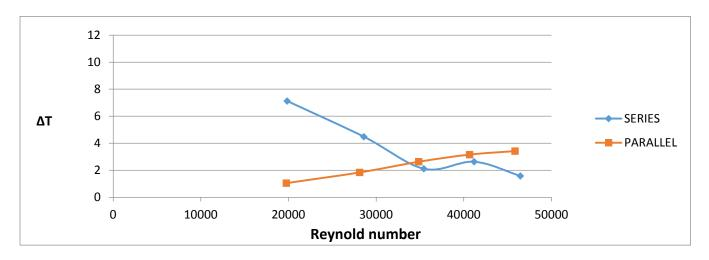
Figure 14. Comparison of temperature difference vs. Reynolds number for both connection
