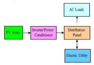
**Figure 2.** Block Diagram of Grid Interfaced PV System
