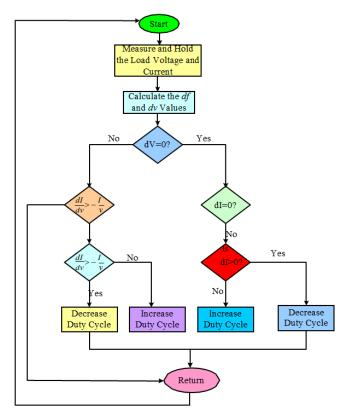
Figure 6. Flow Chart of Incremental Conductance
