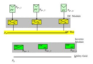
**Figure 8.** Zhang et al. [16] Modular Grid and PV System Configuration
