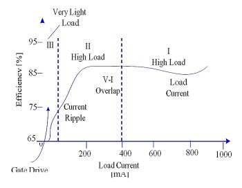
Figure 4. DC-DC Converter Efficiency Curve
