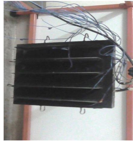
Figure 4. Plain Blackened Vertical Plate with Fins
