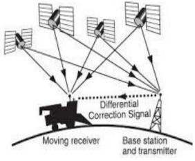
Figure 2 : Real-time differential GPS
