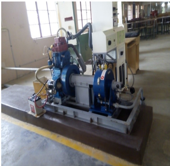
Figure 1. Experimental Setup of VCR Diesel Engine
