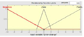
Figure 6: Membership function for delta error
