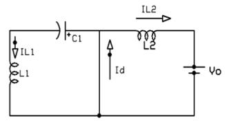
Fig 3: Luo converter with MOSFET OFF condition
