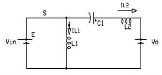
Fig 2: Luo converter with MOSFET ON condition
