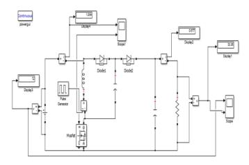
Figure 9: Simulink Model for Luo converter
