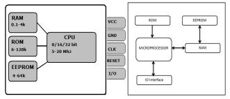
Figure 10: SIM Card structure [17].
