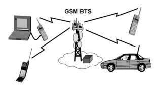
Figure 15: GSM Base transceiver Station.
