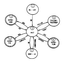
Figure 6: Mealy-Graph for the MS access procedure.
