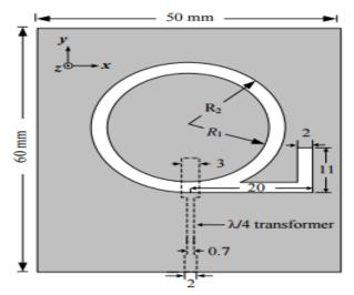
Figure 6. Geometry of proposed ARSA with inverted L-shaped slot
