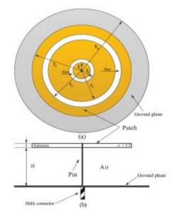
Figure 1. Front view of the Circular Patch Antenna
