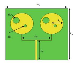
**Figure 3.** A front view of  $2 \times 1$  circular array patch with double circular slots,
