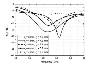
Figure 2. Bandwidth and Return loss performance of the Circular Patch Antenna
