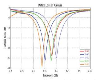
Figure 4. Return loss performance of the  $2 \times 1$  circular array patch antenna with different radius dimension of R1
