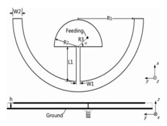
**Figure 8.** Layout of the dual-frequency microstrip antenna of Narrow Half-Ring and Half-Circular Patch
