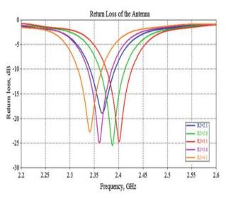
Figure 5. Return loss performance of the  $2 \times 1$  circular array patch antenna with different radius dimension of R2
