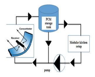
Figure 2. Schematic representation of solar cooking
