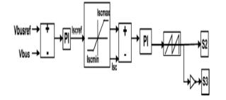
Fig. 5. Modeling of SC Controller
