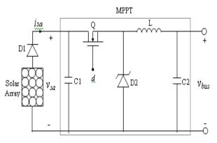
Figure 2. Circuit schematic of the photovoltaic power subsystem
