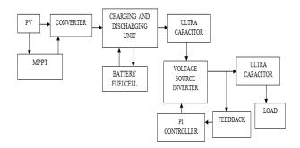
Figure 1. PV-FC-battery-SC hybrid system
