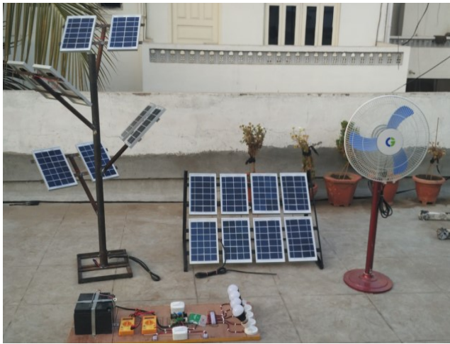
Figure 6: Different Arrangements of solar panels with the control circuit and DC load
