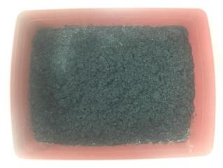
Figure 1: crumb rubber soaked in sodium hydroxide
