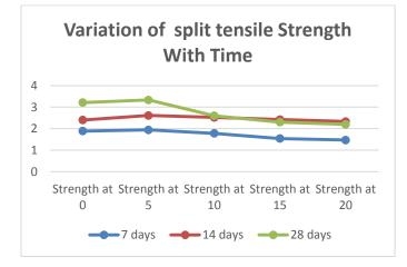
Figure 6: graph showing split tensile results at different days
