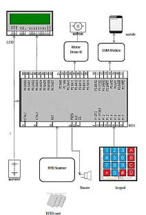
Figure 1. Block Diagram
