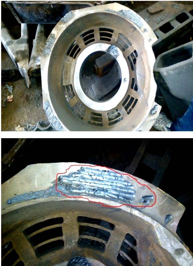
Figure 1. Blow Hole Defect in Bearing Housing
