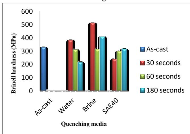
**Figure 3.** Effect of soaking time and quenching media on the hardness of aluminium bronze
