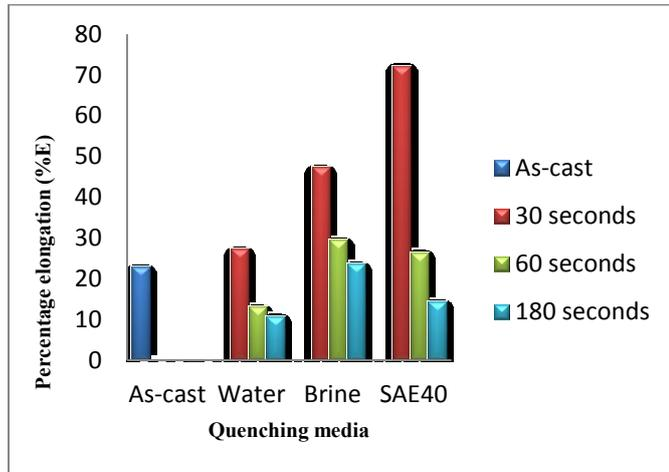
**Figure 1.** Effect of soaking time and quenching media on the percentage elongation of aluminium bronze
