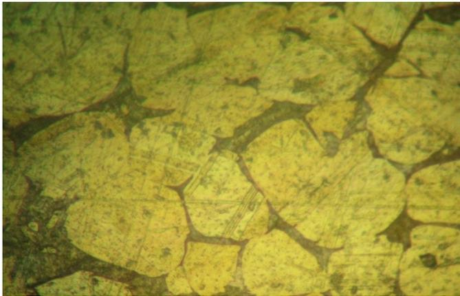
Plate 9. Micrograph of aluminium bronze soaked for 180mins and quenched in SAE 40
