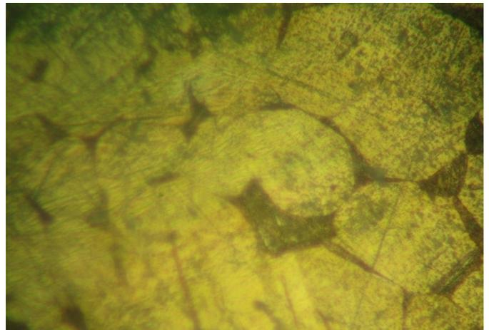
Plate 7. Micrograph of aluminium bronze soaked for 60 minutes and quenched in Brine
