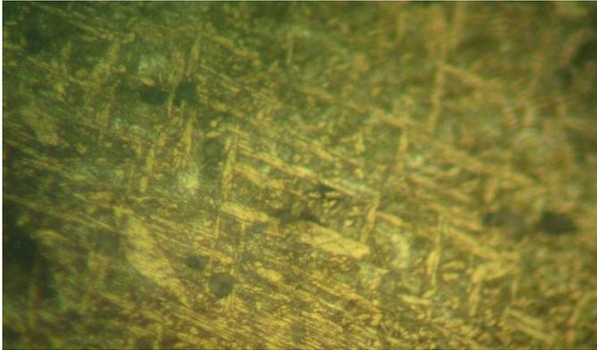
Plate 4. Micrograph of aluminium bronze soaked for 30 minutes and quenched in Brine
