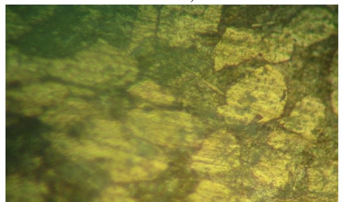
Plate 2. Micrograph of aluminium bronze soaked for 30 minutes and quenched in Water
