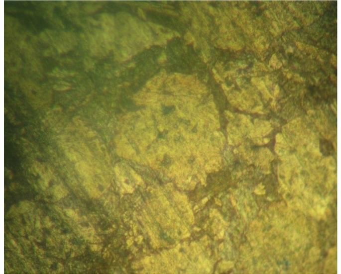
Plate 6. Micrograph of aluminium bronze soaked for 60 minutes and quenched in SAE 40
