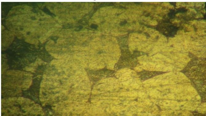
Plate 10. Micrograph of aluminium bronze soaked for 180mins and quenched in Brine
