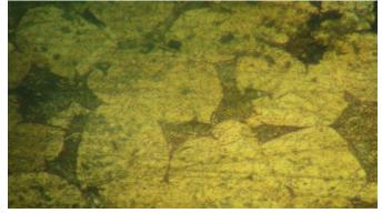
Plate 10. Micrograph of aluminium bronze soaked for 180mins and quenched in Brine
