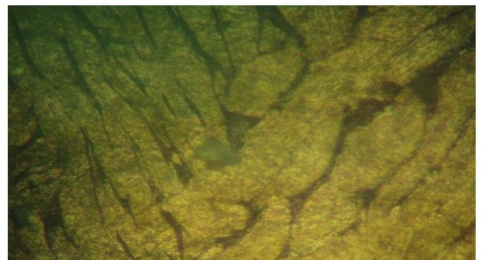
Plate 1. Micrograph of as-cast aluminium bronze (Cu-10%Al)
