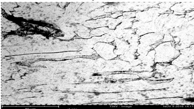
Plate 11. Micrograph (SEM) of Cu-10%Al (As-cast)
