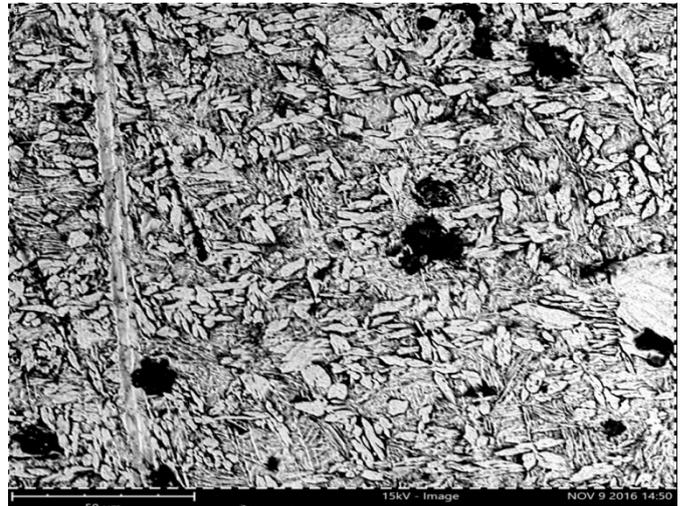
Plate 13. Micrograph (SEM) of aluminium bronze soaked for 30 minutes and quenched in Brine
