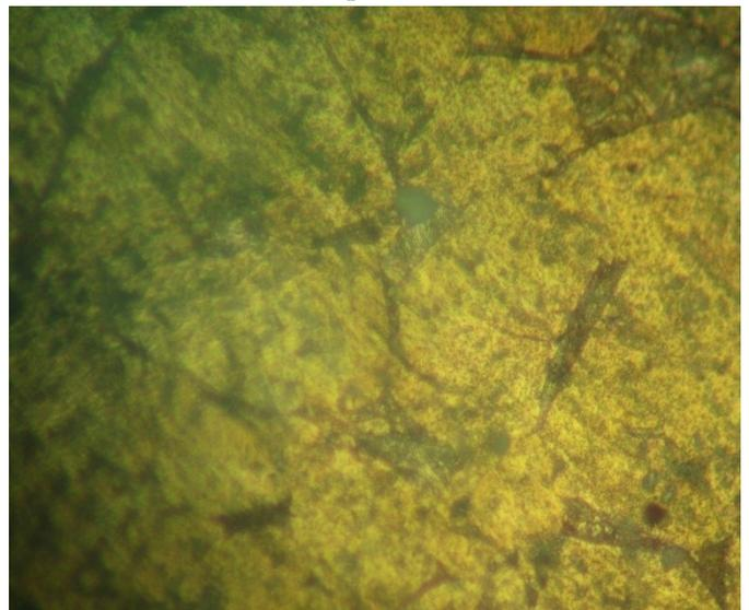
Plate 8. Micrograph of aluminium bronze soaked for 180mins and quenched in Water
