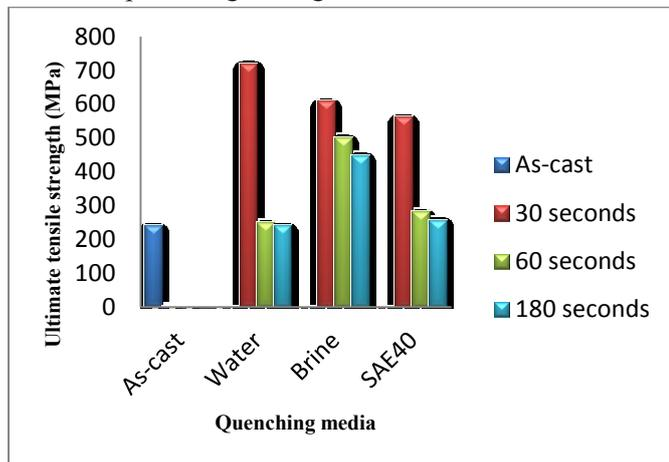
**Figure 2.** Effect of soaking time and quenching media on the ultimate tensile strength of aluminium bronze
