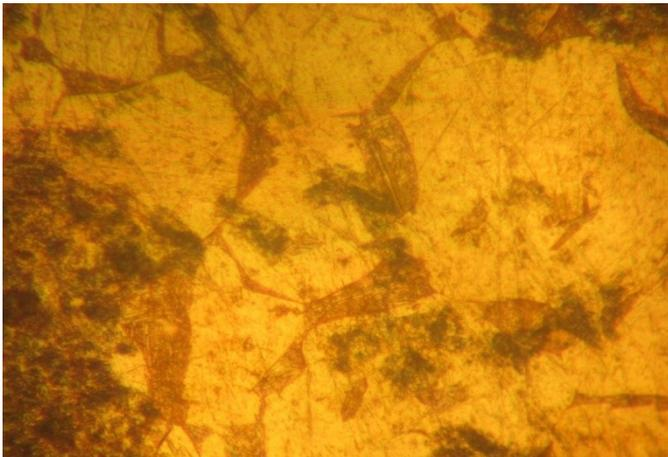
Plate 5. Micrograph of aluminium bronze soaked for 60 minutes and quenched in Water
