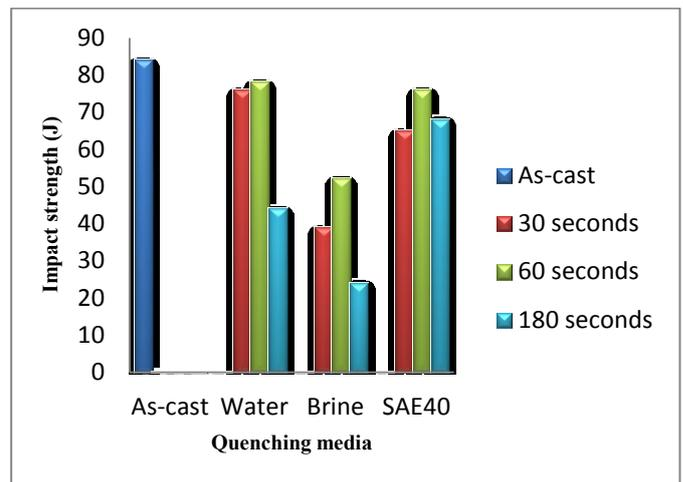
**Figure 4.** Effect of soaking time and quenching media on the impact strength of aluminium bronze
