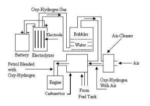
Figure 1. hho generator with engine
