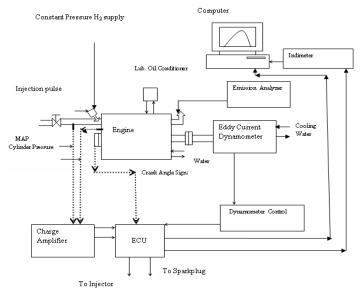
Figure 2. modified hydrogen fuelled engine[4]
